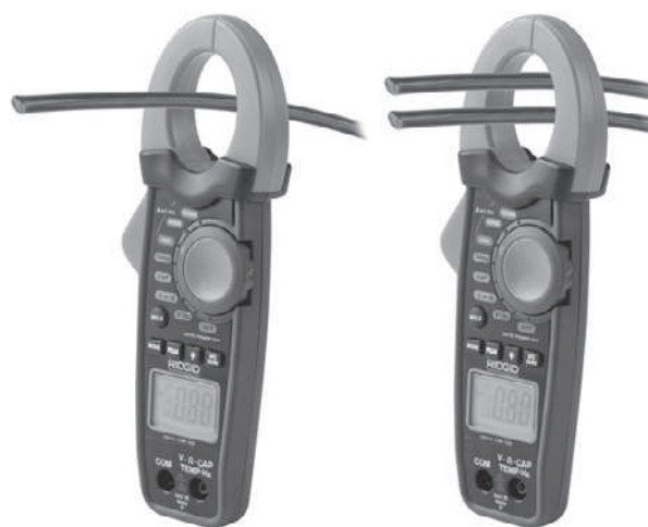
Correct Current Measurement
